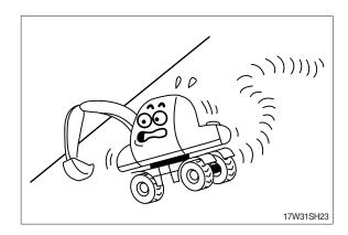
The engine angularity limits are 30 degree. Do not operate by more than the engine limits in any case.
