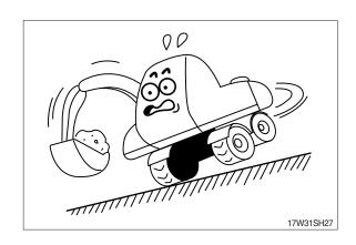
Avoid parking and stopping on a slope. Lower the bucket to the ground and block the tires when parking.
