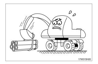
Avoid traveling in a cross direction on a slope as it can cause the danger of rolling over and sliding.
